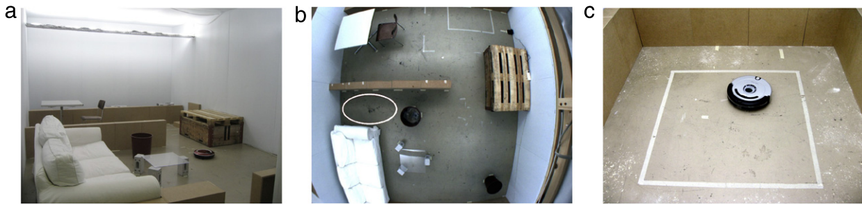
Fig. 3. The experimental setups for the technical study. (a) Arena reproducing an apartment, side view. (b) Arena reproducing an apartment, from the overhead camera. The white ellipse marks an area of difficult access. (c) Simple arena for cleaning tests.
