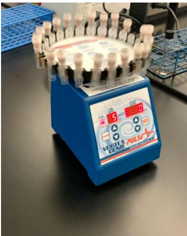
Lysis of bacterial cells to extract DNA using Vortex Genie Pulse.
