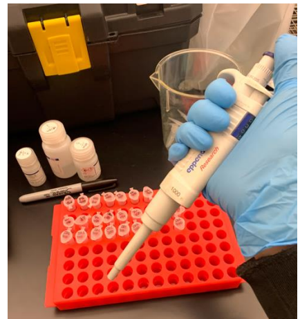
P1000 micropipette used to precisely transfer small volumes of liquids.
